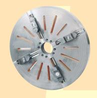
Combo-face plate with four jaws from 32"~60" in diameter
