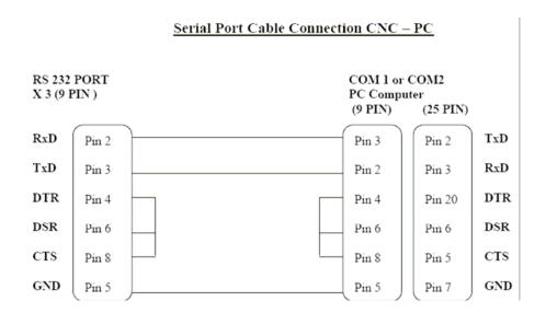
\*\*\*Note: This cable is use for connecting directly from CNC to PC. If you are connecting to Turnkey Package you must use a straight thru cable.
