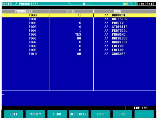
\*\*\*\*Once the parameters have been modified make sure you re-start the control, so the parameters take effect.
