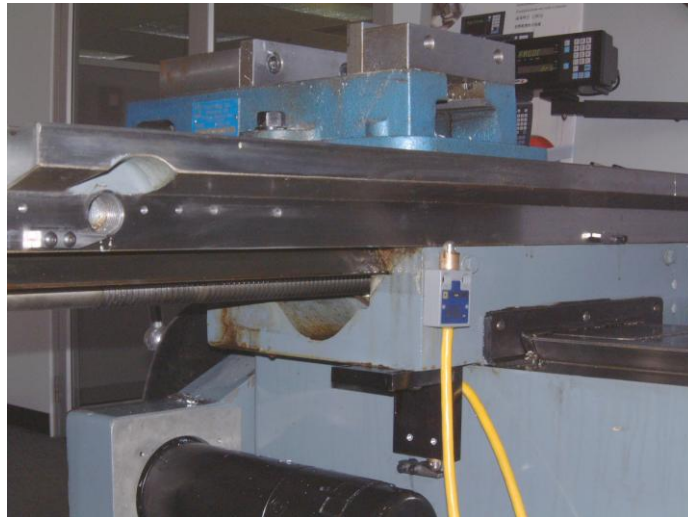
Final installation of switch and two dogs on X axis
