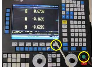
10. Reset spindle and control after mechanical break for tool change or emergency stop.1) Brake spindle. (Fig. 12)
