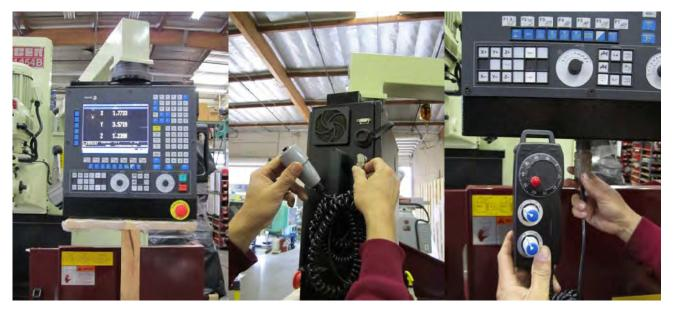
6. Hook up 3 phase power 230V (only) for control power & machine power.
