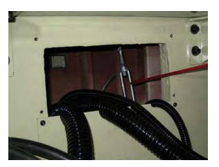
5. Take out control support. Plug in 1. Start/ Stop Push Button Plug 2. Hand Wheel Plug
