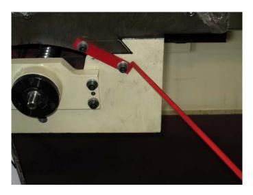
4. Remove the bracket (red) from the Y-axis (in front.)
