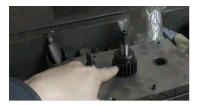
17. Notice the two pins (circled), these are the positioning pin. After taking off the cover, the positioning pin have to be in the same position.
