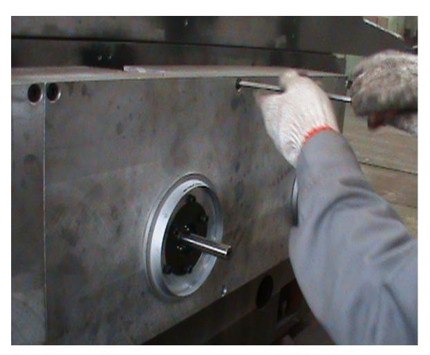
9. When taking off the cover, be careful because the cover is tight and don't damage the shaft.
