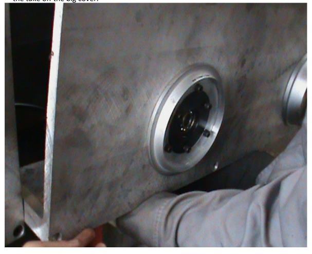
11. After you take off the cover, you will see the gearbox, before you loosen off the screw, you will need to make a mark so when you install it back, every position is the same.
