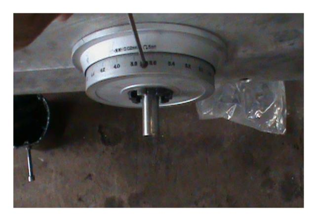
3. Loosen up set screw, take off the clutch.
