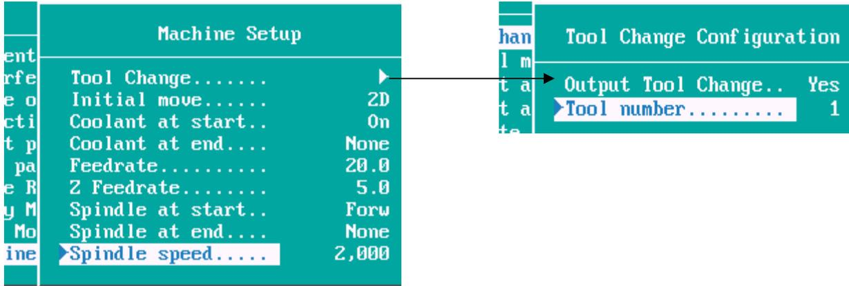
Coolant turn ON at start but not OFF at end as the same tool will be used for pocketing and contouring. The same applies with spindle.
