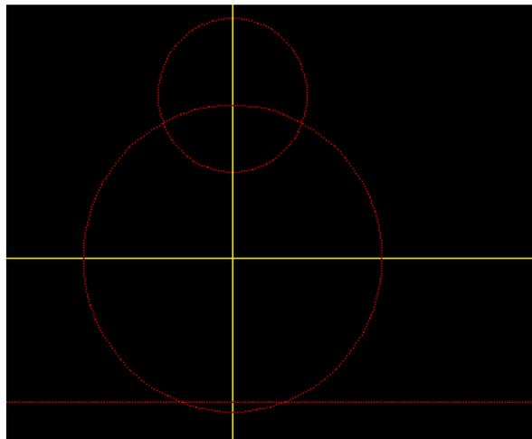
The next geometry required are two points at the intersect of the 4" radius circle and the -3.75 line. To do this use icon circled below.
