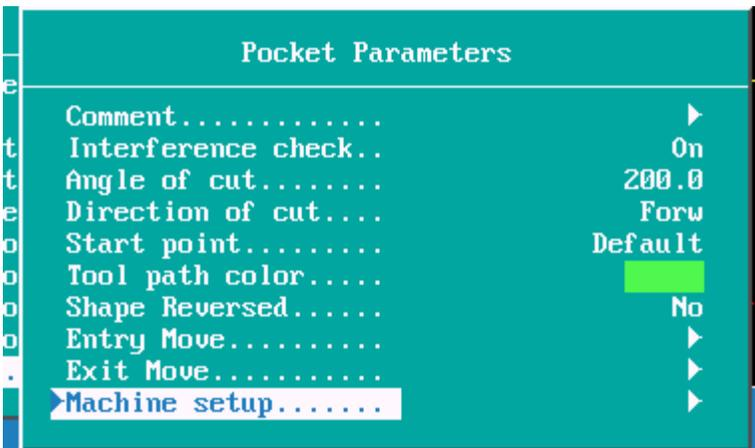
Angle of cut can be left at default or an angle entered, on this part an angle of 200 deg's will be entered.
