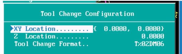
If machine has a tool changer arrow down to Tool Change press enter arrow down to Tool Change Format if M06 is required it should read as follows **T%02DM06**.
