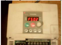
21. Press "▲" 4 times or until LCD displays "F601" and press "ENT" key. Use "▲▼" key to change the number to "150" (If used for heavy cut, change up to 180) and press "ENT" key.
