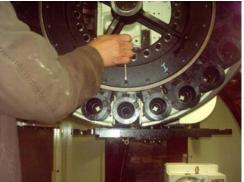
4. Push the pot forward inner side and take the pot upward, then extract it.
