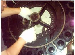
9. Check the correct angled 90 degree with the replaced pot.
