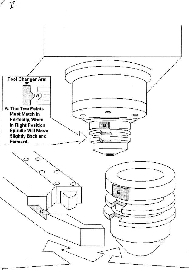
Note: Position Point B in perfect conjuntion with Point C. When Point B and Point C in properly engaged tightly, you can slightly shift the tool left to right by applying a little force. Make certain that Point A (in the above diagram) is fitted perfectly. Point A must be perfectly fitted in order to prevent any tool changer damage. If you have any question please contact ACER.
