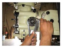
3. Until proper tension is reached, retighten two screws. (Warning: Tension cannot be too high!) Otherwise, quill will return too fast, either the handle will hurt people or it will cause damage on the Reverse Trip Ball Lever and also cut down the life of the clock spring.
