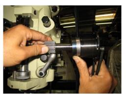
4. Uses dead end hammer to tap clock spring to housing. Align the clock spring to the spring cover slit.
