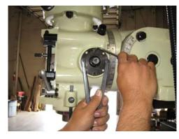
3. Rotate spring cover counterclockwise from head and remove clock spring from housing.
