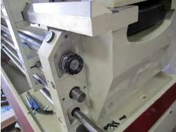
8. Move the apron away from the saddle to disconnect the leadscrew and feed rod.
