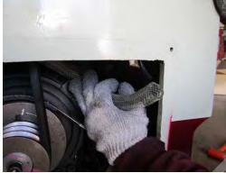
13. Loosen the four gear box fixed screws; (use a lot of force because it is tightly locked.)
