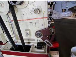
11. Take out the gearbox cover and make three marks for the gear change position.
