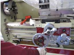
(After disconnecting leadscrew and feed rod)
