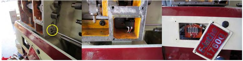
17. Lower down the support screw and take out the gear box.
