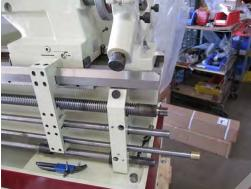
9. Take out the first and second gear from gear box.
