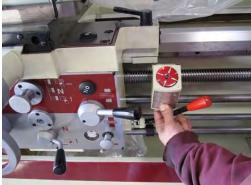
6. Slide out the stop and go rod and 4 way position stop rod.
