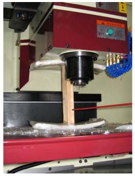
9. Assemble the way cover and coolant pipe.(Make sure the left & right way cover is put on the machine correctly)!
