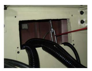
5. Loose M8 Screw on control panel and turn it around.
