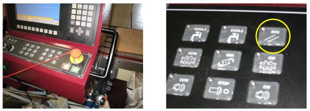
Using the MPG and select one thousands (10). Slowly move the Z up. Remove the Spindle head support. Move the Z down. The counterbalancing weight should be up. Remove the bar.
