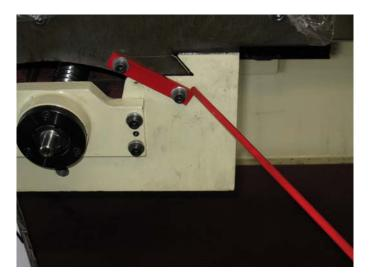
4. Remove the bracket(red) from the Y-axis(in front.)
