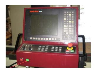
Wait until the control boots up. Release Emergency button. Press the Servo On button (SVO). Select Handwheel (F10).
