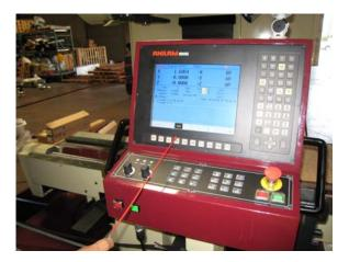
Type "M60" and push the execute (activate) button. Push the magazine rotate button "CW", make sure magazine rotates clockwise.
