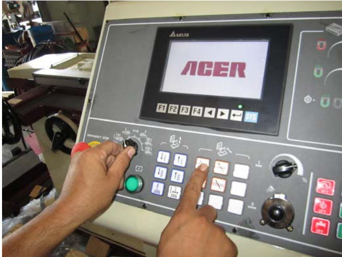
Fig. 8 Make sure table crossfeed moving direction is correct.
