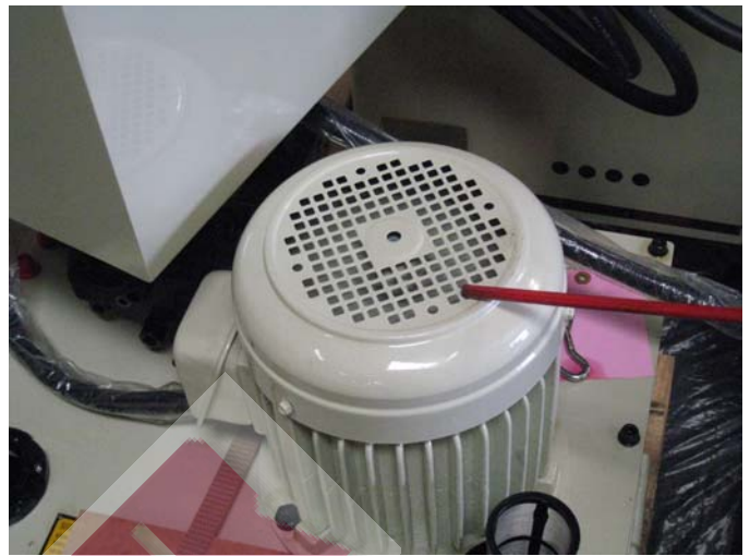
Fig. 5 Make sure hydraulic motor rotation is clockwise.
