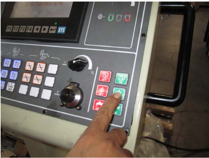
Fig. 6 Make sure the dust collector motor is running.
