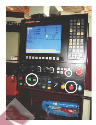
8. Check rotation of magazine by pushing magazine counterclockwise and clockwise buttons.
