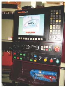
Person A, who is on the ground release emergency push button and press "SERVO RESET" and turn control function to Z, and set Feed to 10%, & jogging + sign to raise up spindle head high enough to remove the support.
