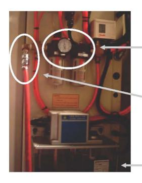
Pull knob up and turn to adjust setting. 90 psi minimum
