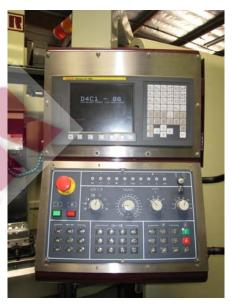
Turn function knob to hand wheel function (See page 4) (HND) on display. Select Z on MPG (Manual Pulse Generator). Set to X100, slowly move up spindle (+) and take out spindle support (orange bracket)
