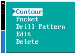
The first tool path is **pocket** using arrow keys high light pocket press.
