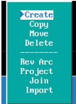
A start point needs to be established for are shape, high light will be on **Create**. Create will set where the shape is going to start.
