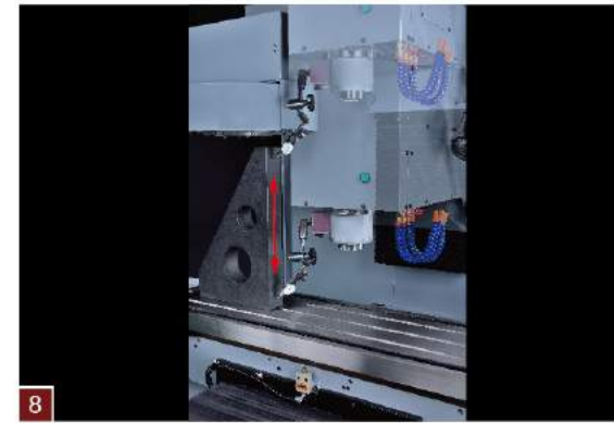
8 Squareness of the head movement to the table is measured at two viewpoints. Measurement of Z to X plane and Z to Y plane has an allowable number of 0.0004" per 12".
