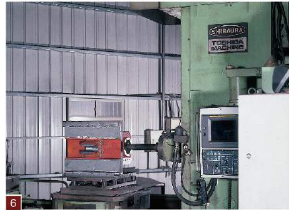
6 With a special fixture on a horizontal boring machine, the spindle housing is machined and honed to within 0.0002" per 12", and its parallelism to the guideway is within 0.0004" per 12".
