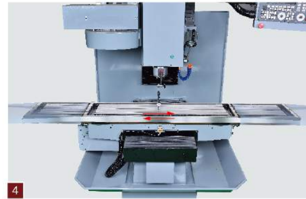
4 Parallelism of the table movement in X axis is dial in with a dial indicator. The permissible value is 0.0004" per 20".
