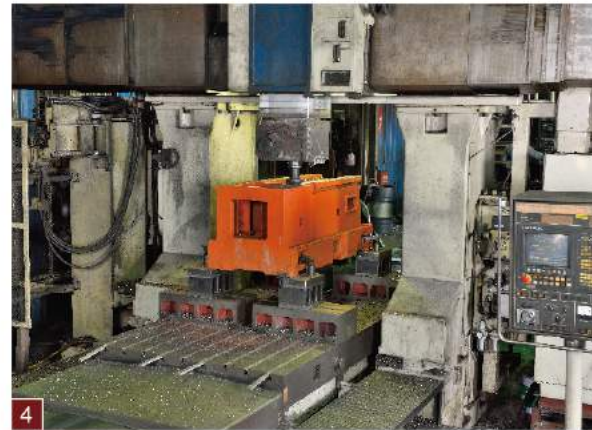
4 The final foundation of accuracy (squareness, flatness, and parallelism) is milled and machined exclusively on a five-face machining center. The accuracy is guaranteed to be within 0.0004" of each overall travel axis.
