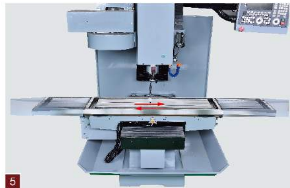
5 Parallelism of the T slot and X axis movement is also an inspection value. Normally per 40" the tolerated maximum number is 0.0008".
