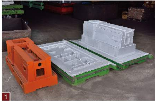
1 A great form casting comes from a precision crafted mold. For its outer appearance, ACER iron castings are vividly recognized from the molds and at the machining sections, they are precisely casted within 5mm of finished dimension. This enables a fast, clear and precision machining done within a specified time.
