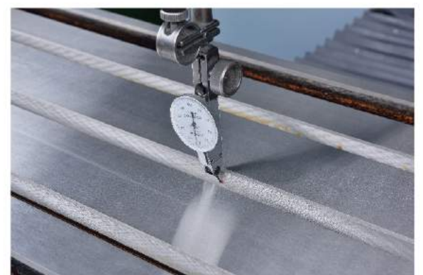
5 Parallelism of the T slot and X axis movement is also an inspection value. Normally per 40" the tolerated maximum number is 0.0008".
