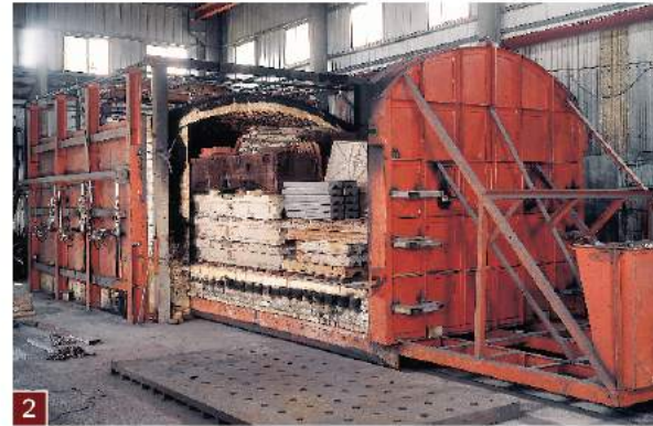
2 The exceptionally high-stiffness "MEEHANITE" casting undergoes an annealing process to eliminate internal stress prior to machining.
