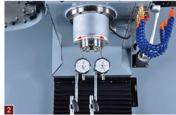
2 Axial run-out of the spindle is measured and recorded. Less than 0.0002" is the permissible value.
