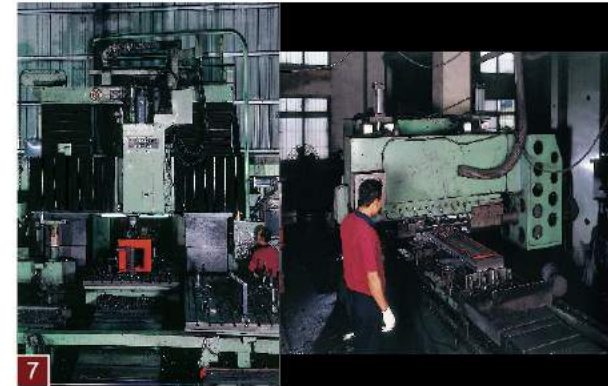
7 Specially designed bridge-type planer mills are used to machine ACER working tables and columns. The parallelism of the slideways to each other and the T-slots to the guideway are guaranteed to be within 0.0008" of each other.
