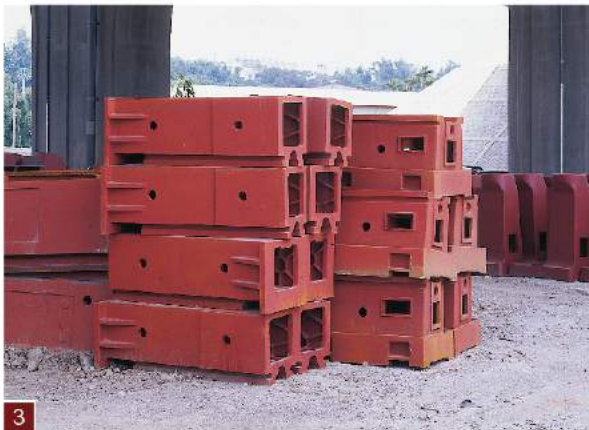
3 All annealed ACER FC-30 iron castings are stockpiled and aged prior to machining. This is done to eliminate future molecular realignment and deformation on the castings.
