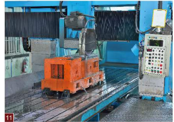
11 The base of the machine is the foundation of a machine's accuracy. The slideways on the base of ACER bed mills are hardened and ground to within 0.0004" over the entire travel length.
