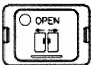
Manual Door Interlock Released Function Key with the LED
