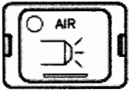
Manual Work Pieces Air Blasting Function Key with the LED
