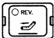
Manual Chip-Conveyor CW, CCW Turning Function Key with the LED
