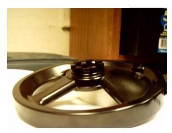
3<sup>RD</sup> GENERATION HANDWHEEL WITH CLUTCH, 7 TEETH 19.7 MM INSIDE DIAMETER
