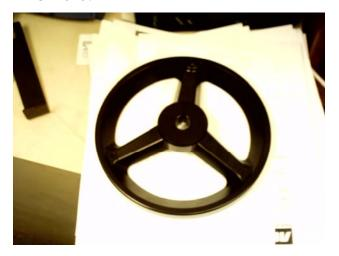
1<sup>ST</sup> GENERATION HANDWHEEL NO CLUTCH 17 MM INSIDE DIAMETER
