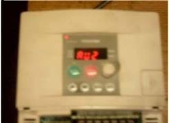
24. Press "MON" key until LCD displays "AU1" and then use "▼" key to find "F---" and press "ENT" and LCD should display "F100". Use "▼" key to find "F700" and press "ENT" key. Use "▲ ▼" key to change number to "1" and press "ENT"
