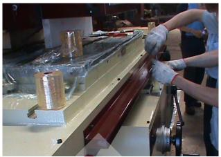
Then remove the travel rail (just lock it directly when putting it back, there is no positioning problem.)
