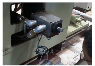
This type of hydraulic pipe only needs to remove the two pipes A and B, and they will be marked with a nameplate.
