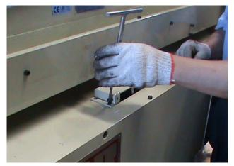
The removed reversing induction seat is plugged back into the inside and fixed together after the oil pressure valve cover is removed.
