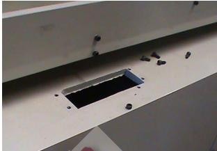
Remove the hydraulic valve crank and cover
