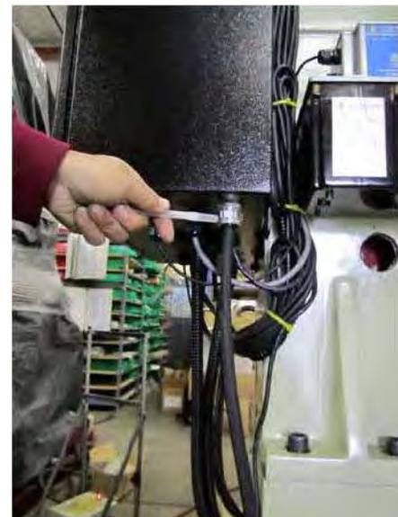
5. Release Emergency Stop button. Toggle function switch to “Man”. Turn on spindle Forward/Reverse Switch. Check spindle rotation. Make sure it is correct. If opposite direction, please turn off main power by pushing emergency button. Switch any two power lines that go into the machine.
