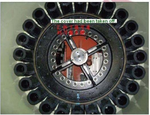
3. You will see the Cam Shaft (an area with grease on the upper left side of the ATC).
