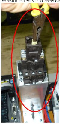
After opening the eletric cabinet door, please use a needle nose pliers to turn the power to PLC unit.
