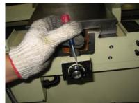
12. Punch one spike of the spring washer back to the lock washer setting grove.
