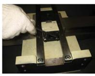
6. Loosen four M6 screws. Take out shaft bush.
