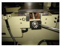
10. Put back spring washer face outwards. Put back second locking nut.
