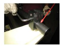
20. Connect the connecting rod to the shaft. Tighten the M6 screw when using taper turning attachment.
