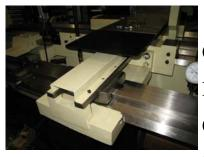
18. Tighten eight M5 screws on cover of the taper turning attachment. Put back the cover of the cross slide by tighten three M5 screws.
