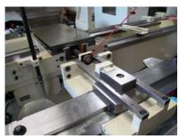
14. Bring in the taper turning attachment and align it with the screw and the body of the taper turning attachment.
