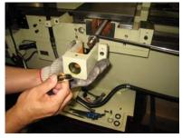
4. Slide out bracket. Take off bearing on crossfeed screw bracket. Keep support bearing.
