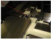
17. Use dial indicator to align the level of the slide place. Move the apron 8 inches left or right to make sure it is zero to zero. (Adjust the
