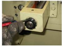
2. Loosen first locking nut. Then loosen the spring washer, take off second locking nuts.
