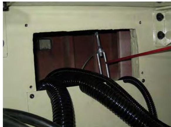
5. Take out control support. Plug in 1. Start/ Stop Push Button Plug 2. Hand Wheel Plug
