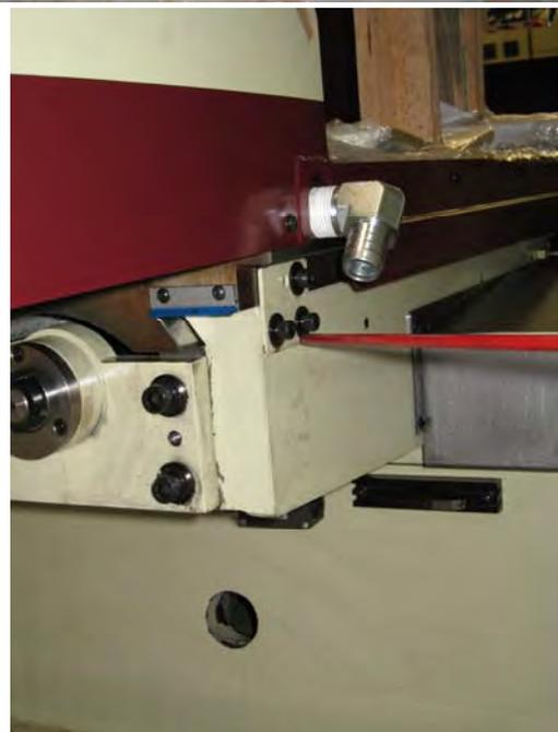
4. Remove the 4 screws on the back cover. Loose the 2 locks on both end of the double nut clamper. Twist the center to remove the clamper. Then take out the hook attached to the counter weight inside column.
