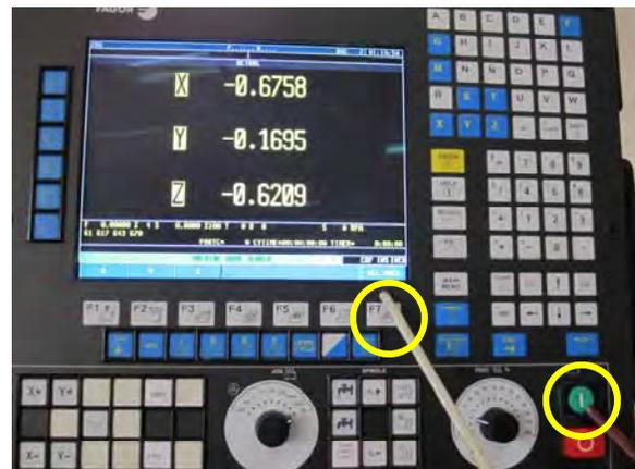
10. Reset spindle and control after mechanical break for tool change or emergency stop.
