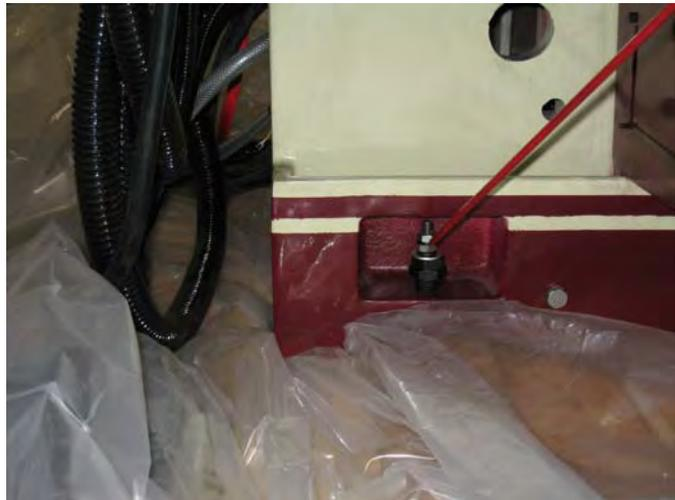
3. Remove the 3 M8 screw on the bracket on the X-axis (facing machine's
