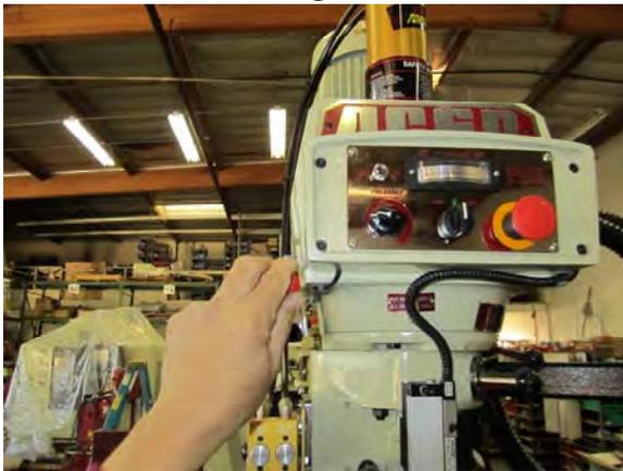
2) Toggle spindle Forward/Reverse Switch to neutral; then switch to forward or reverse, spindle is turning.
