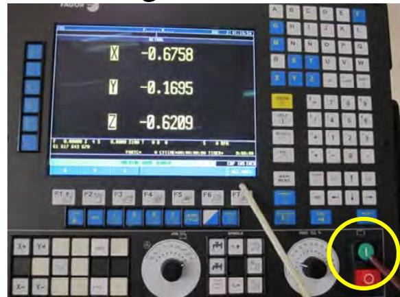
Type "S1000M3". Press the Execute button (Fig. 18). Spindle start running. Then press Spindle Stop. Press Spindle Forward. Then press Spindle Stop. Press Spindle Reverse. Always press Stop before changing spindle direction. (Fig. 19).
