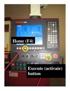
Type "M60" and push the execute (activate) button. Push the magazine rotate button "CW", make sure magazine rotates clockwise. If not, change power source direction by swapping any of the two of the three power wires.
