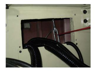
5. Loose M8 Screw on control panel and turn it around.
