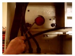
8. Assemble the splash guard and way cover.
