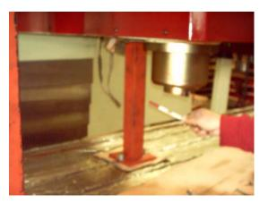
spindle head support. Move the Z down. The counterbalancing weight should be up. Remove the bar.
