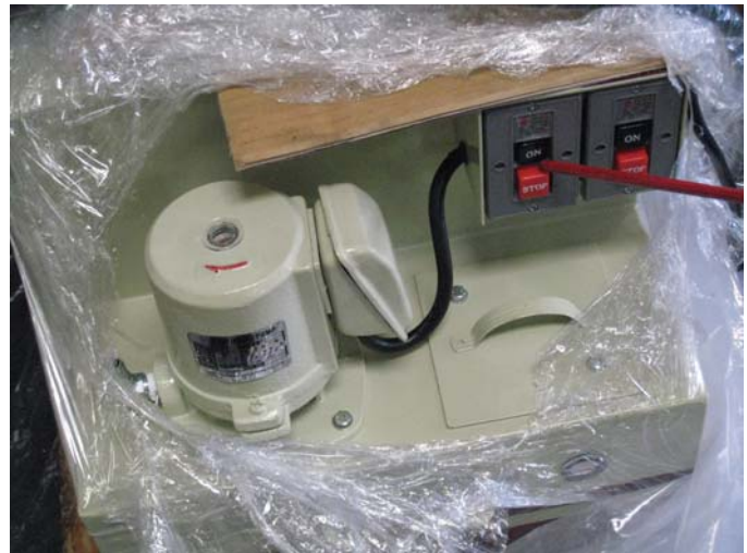
Fig. 7 Make sure the coolant pump is running clockwise.
