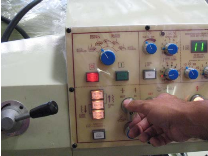
Fig. 9 Make sure Rapid Up/Down direction is correct.
