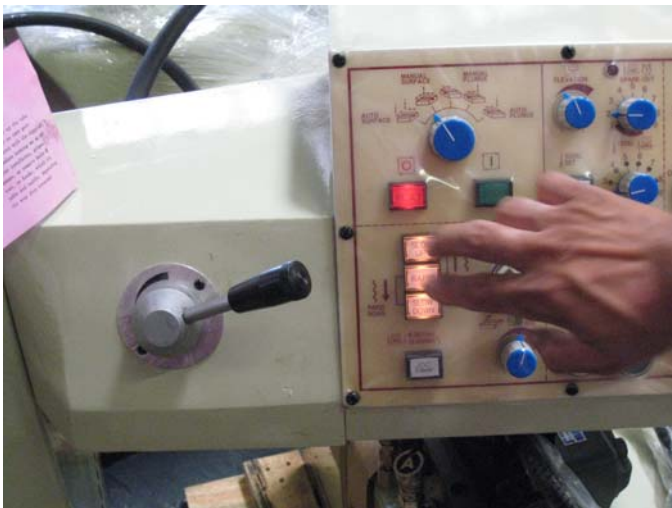
Fig. 9 Make sure Rapid Up/Down direction is correct.
