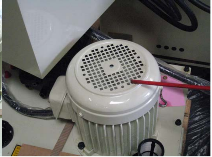
Fig. 5 Make sure hydraulic motor rotation is clockwise.
