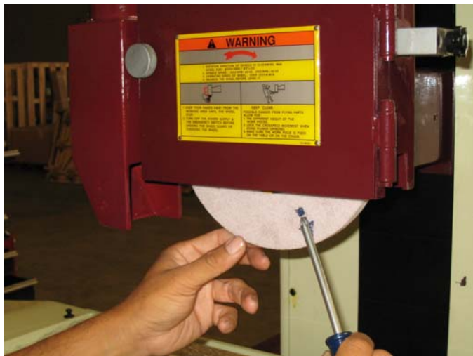
Fig 2. Tap wheel with an object. Make sure the wheel is not cracked. The sound should be clear and consistent.
