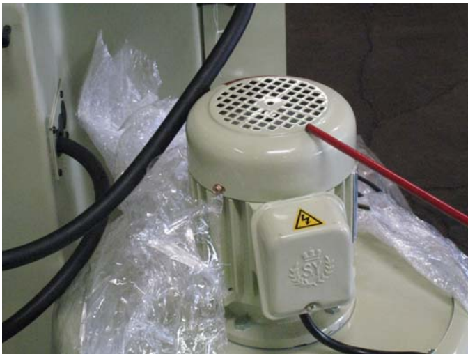
Fig. 6 Make sure the dust collector motor is running clockwise.
