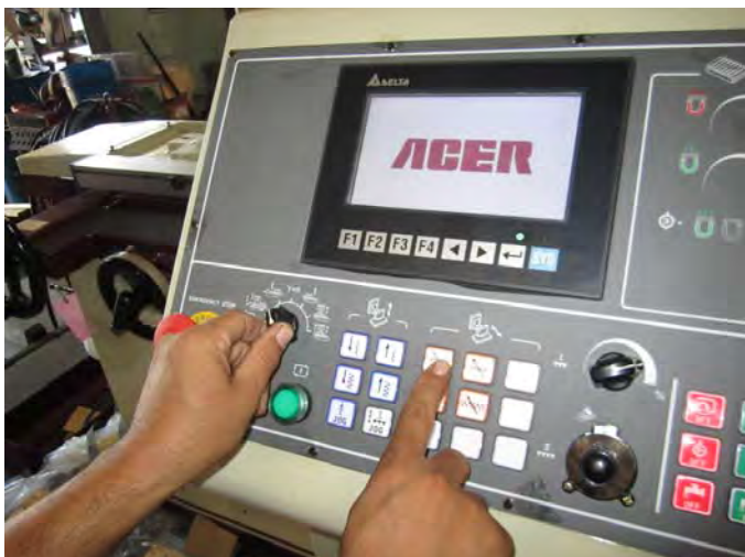
Fig. 7 Make sure table crossfeed moving direction is correct.
