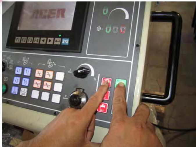
Fig.3 Push On and Off immediately. Make sure spindle rotation is clockwise.
