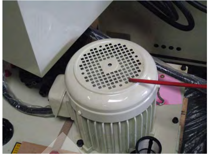
Fig. 5 Make sure hydraulic motor rotation is clockwise.
