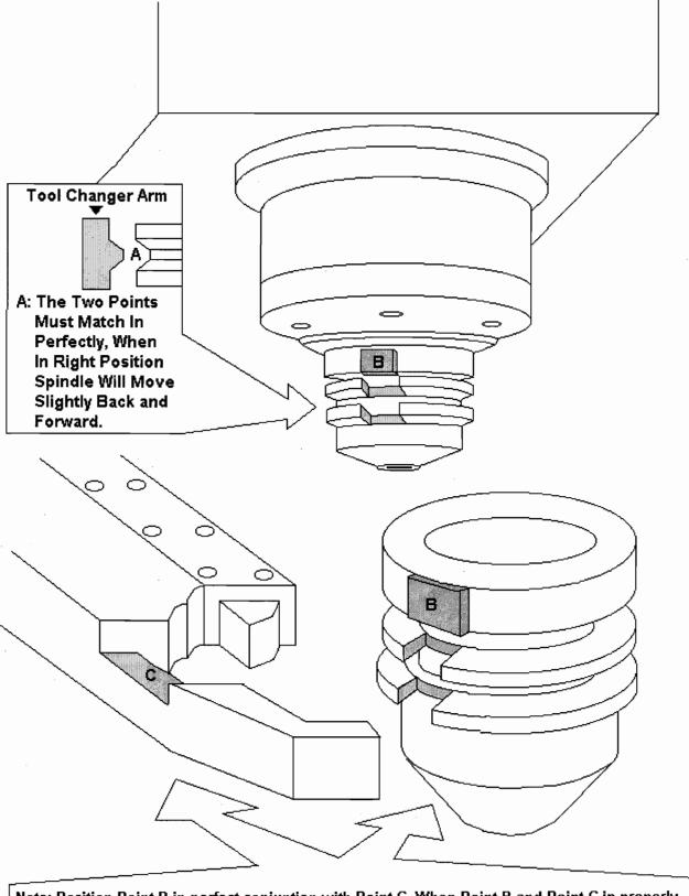
Note: Position Point B in perfect conjuntion with Point C. When Point B and Point C in properly engaged tightly, you can slightly shift the tool left to right by applying a little force. Make certain that Point A (in the above diagram) is fitted perfectly. Point A must be perfectly fitted in order to prevent any tool changer damage. If you have any question please contact ACER.
